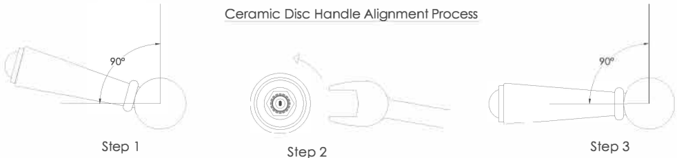
Ceramic Disc Handle Alignment Process
